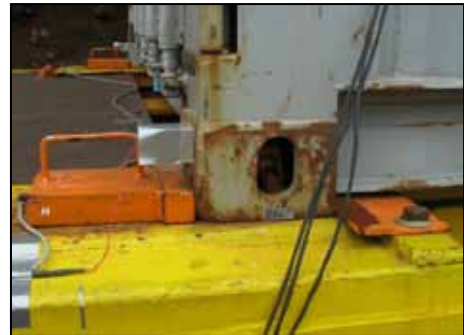
Figure 7: Distance between marks on the diagonally opposite corner castings
