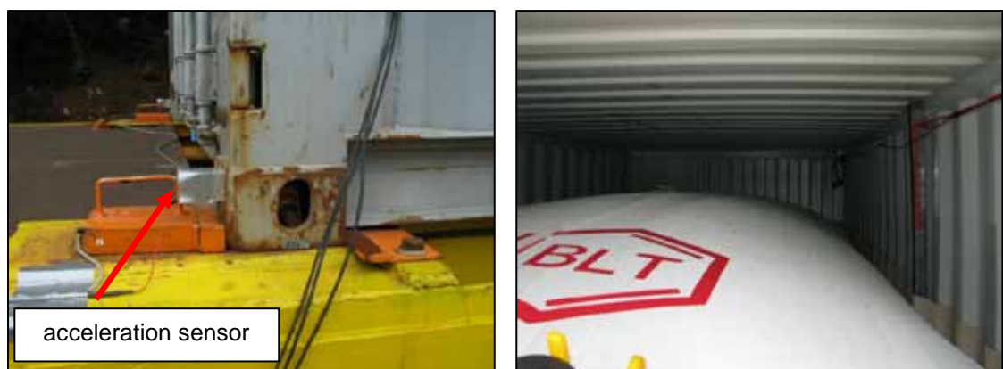
Figure 1: Container barriers and acceleration sensors / view on Flexitank
