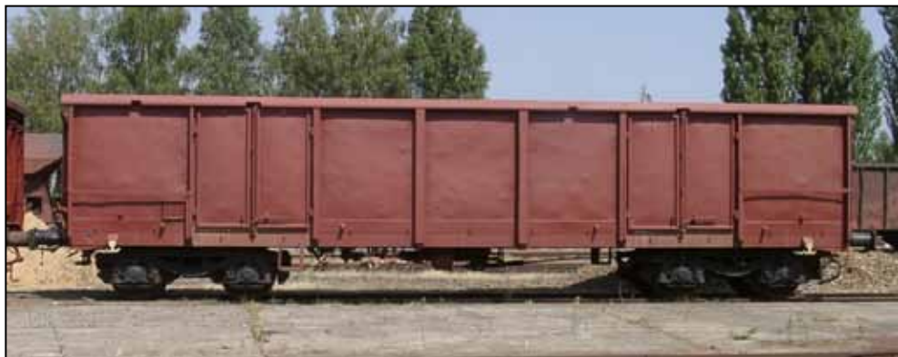
Figure 13: Impact wagon according to ERRI, no. 14 (80 t) loaded with standard UIC ballast
